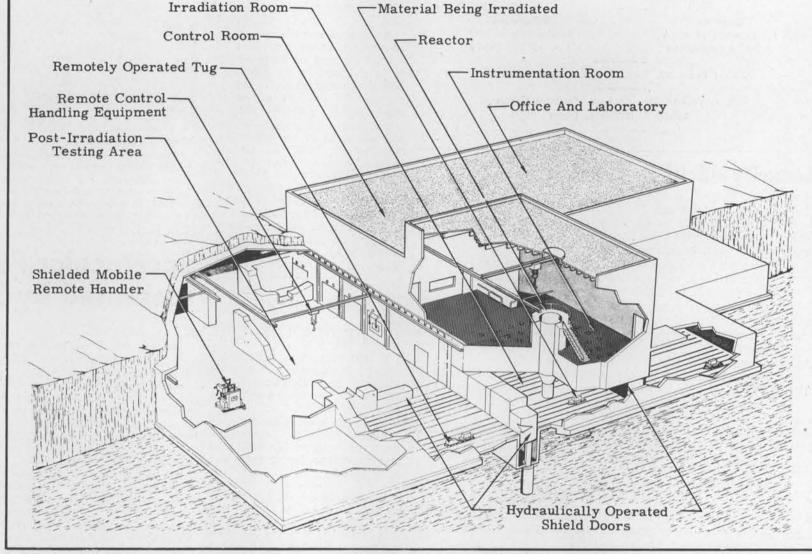
PROPOSED Sandia Engineering Reactor Facility (SERF) for Sandia Corporation engineering testing work is shown here in an artist's
